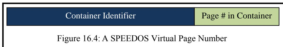
In the MONADS systems the ATU actually achieved the equivalent of this. Each virtual address in the MONADS local area network was unique, and David Abramson designed an ATU, based on a hash table implemented in hardware, which could translate any virtual page number in the network to a page frame number (or cause a page fault interrupt) [95].
